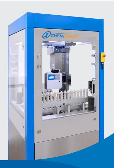
Chemspeed's FLEX POWDERDOSE with its proprietary overhead gravimetric solid dispensing / dosing (mg to g) and our user-friendly software allow you to automatically dispense virtually any powder / solid and extrudate into any type of destination.
